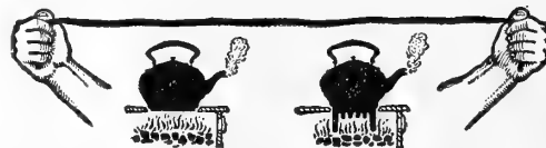
These sketches, go to prove that a kettle with a corrugated or looped bottom has the same quick heating space that a flat bottomed one has, three times the width. On this fact is based the use of corrugations in the fire box top of greenhouse boilers
